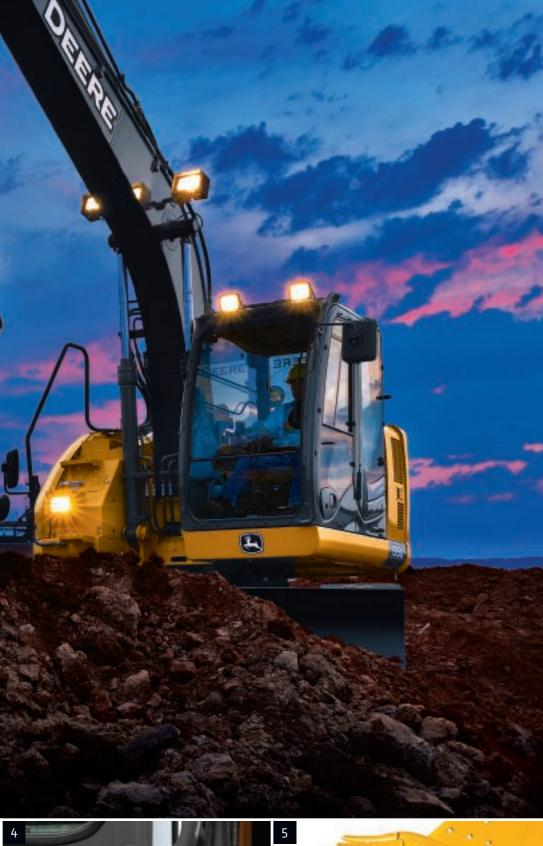
A John Deere exclusive, three welded bulkheads within the boom resist torsional stress for unsurpassed durability. Booms, arms, and mainframes are so tough, they're warranted for three years or 10,000 hours.
