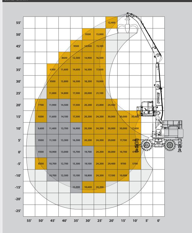
Attachment weight is to be deducted from the values to get lift capacity (values represent load on yoke) Values are in lbs and conform to ISO 10567 and ASME B30.25
