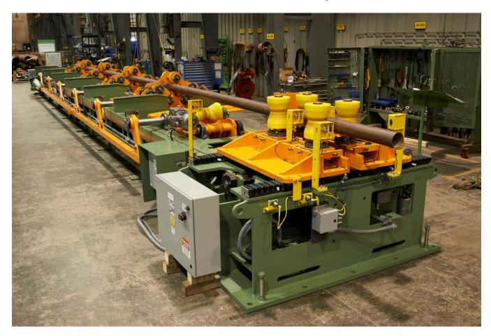
The Brandt Thread Table utilizes adjustable stops to position one pipe at a time on the table. The table is designed with four independent idler rolls used to absorb vibration while the pipe is spinning during the
