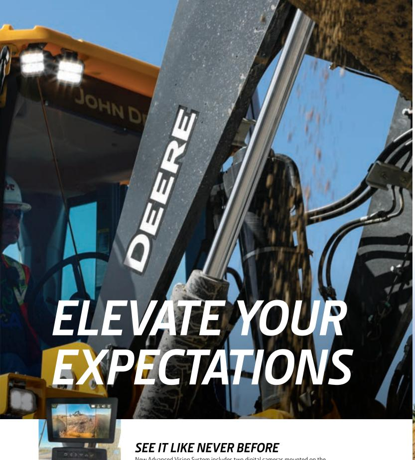
New Advanced Vision System includes two digital cameras mounted on the rearview-mirror platforms that integrate with the rearview camera for a single display on a dedicated in-cab monitor. Overlayed within the monitor's rear-camera view, dynamic reversal projected-path lines help operators visualize the loader's anticipated reversal path based on its articulation, for sight lines to people or objects directly within the path.
