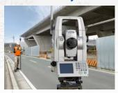
The NET Series offers high-precision angle accuracy (NETO5 AXII: 0.5", NET1 AXII: 1"), which can be applied for a wide range of precise measurements. The high-precision 3D station is equipped with an automatic tracking system and can be configured by remote control.
