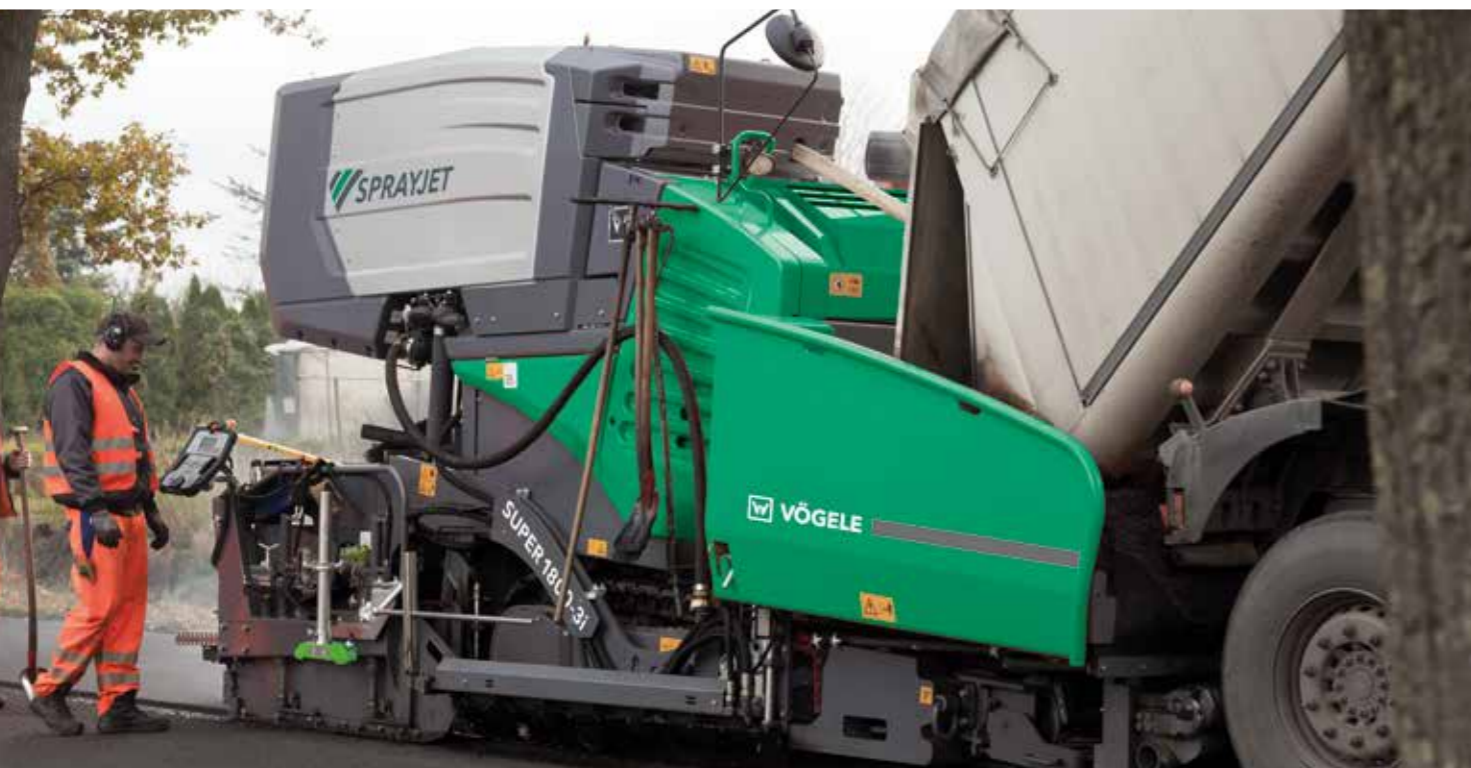
The power unit of the SUPER 1800-3i SprayJet with diesel oxidation catalyst (DOC) and selective catalytic reduction (SCR) for exhaust gas after-treatment complies with the strict requirements of European exhaust emissions standard Stage 4 and US EPA standard Tier 4f.
