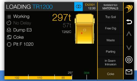
The iVolve screen displays load pass and total tonnage, BCM, material, location and centre-of-gravity data directly to the excavator (or loader) and truck operators via an in-cab screen, assisting optimal loading of every truck.
