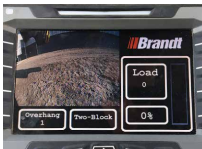
Counterweight-side camera view with additional lift details
