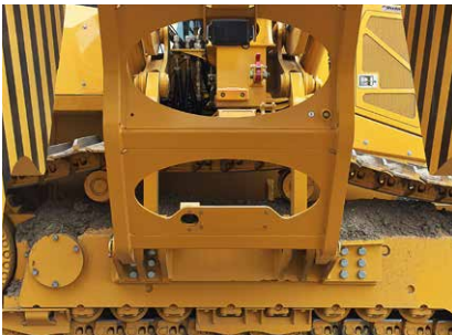
Concealed counterweight-side camera and radar
