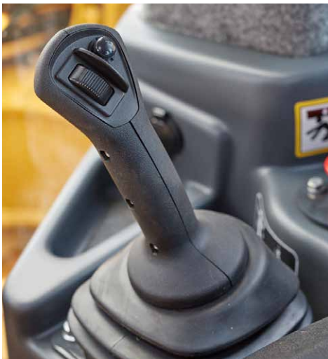
Electro-hydraulic sideboom control joystick
