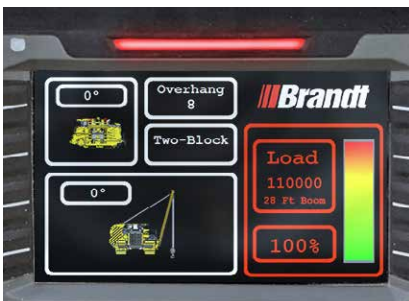
Red with buzzer indicates load limit reached
