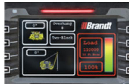
Red with buzzer indicates load limit reached
