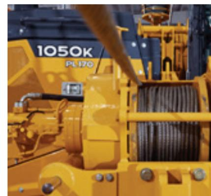
Boom side load winch (left side)
