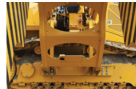
Concealed counterweight-side camera and radar
