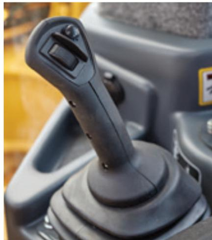
Electro-hydraulic sideboom control joystick
