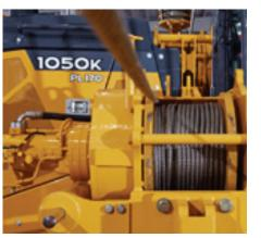
Boom side load winch (left side)
