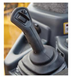
Electro-hydraulic sideboom control joystick
