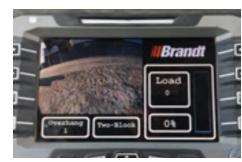
Counterweight-side camera view with additional lift details
