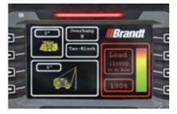
Red with buzzer indicates load limit reached
