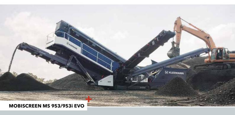
The mobile screening plant MOBISCREEN MS 953 EVO is equipped with a  $9.5 \, \mathrm{m}^2$  screen box. The triple-deck screening plant impresses with a feed capacity of up to  $500 \, \mathrm{t/h}$ . It is operated by a modern control system. All functions are thus easy to control, operating statuses and machine functions can be viewed at any time.
