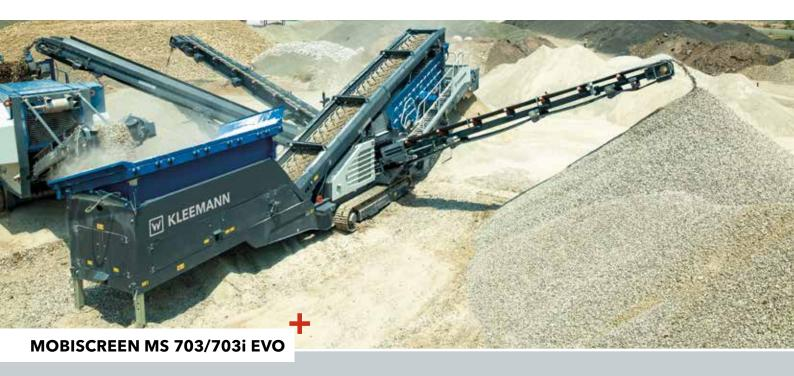
The mobile screening plant MOBISCREEN MS 703 EVO is equipped with a 7 m2 screen box and is used as a double-deck classifying screen. The plant is characterised by favourable transport dimensions and shut setup times. The screen plants are operated by a modern control system. All functions are thus easy to control, operating statuses and machine functions can be viewed at any time.
