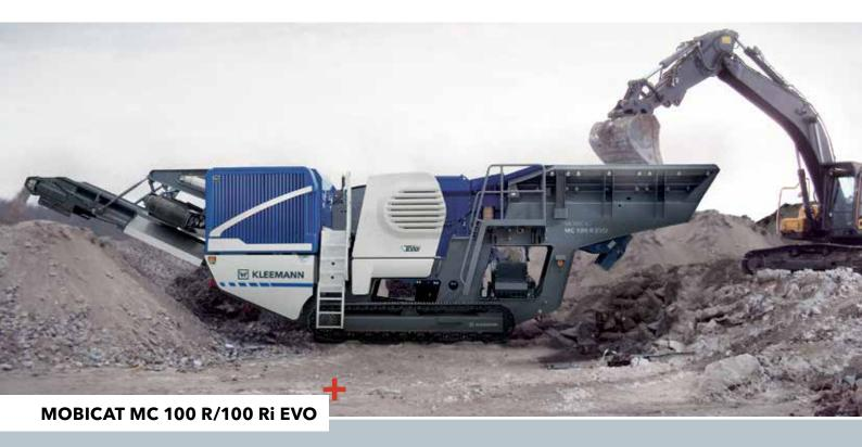
The smallest mobile jaw crusher in the EVO range is impressive thanks to its compact design and reliability. It can be used for a huge variety of materials, offering wide-ranging possibilities for both demolition companies and contract crushers. The MC 100 R EVO is economical to use thanks to its diesel-directdrive.
