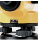
for protection against dirt and scratch. The readout window is located below the eyepiece for quick reading.
