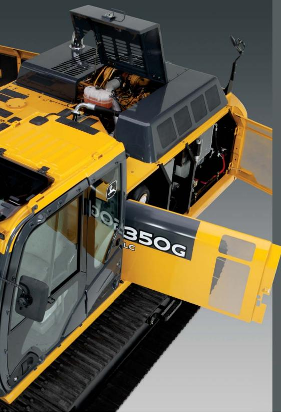
Large fuel tanks and 500- and 5,000hour engine and hydraulic oil-service intervals decrease downtime for routine maintenance.
