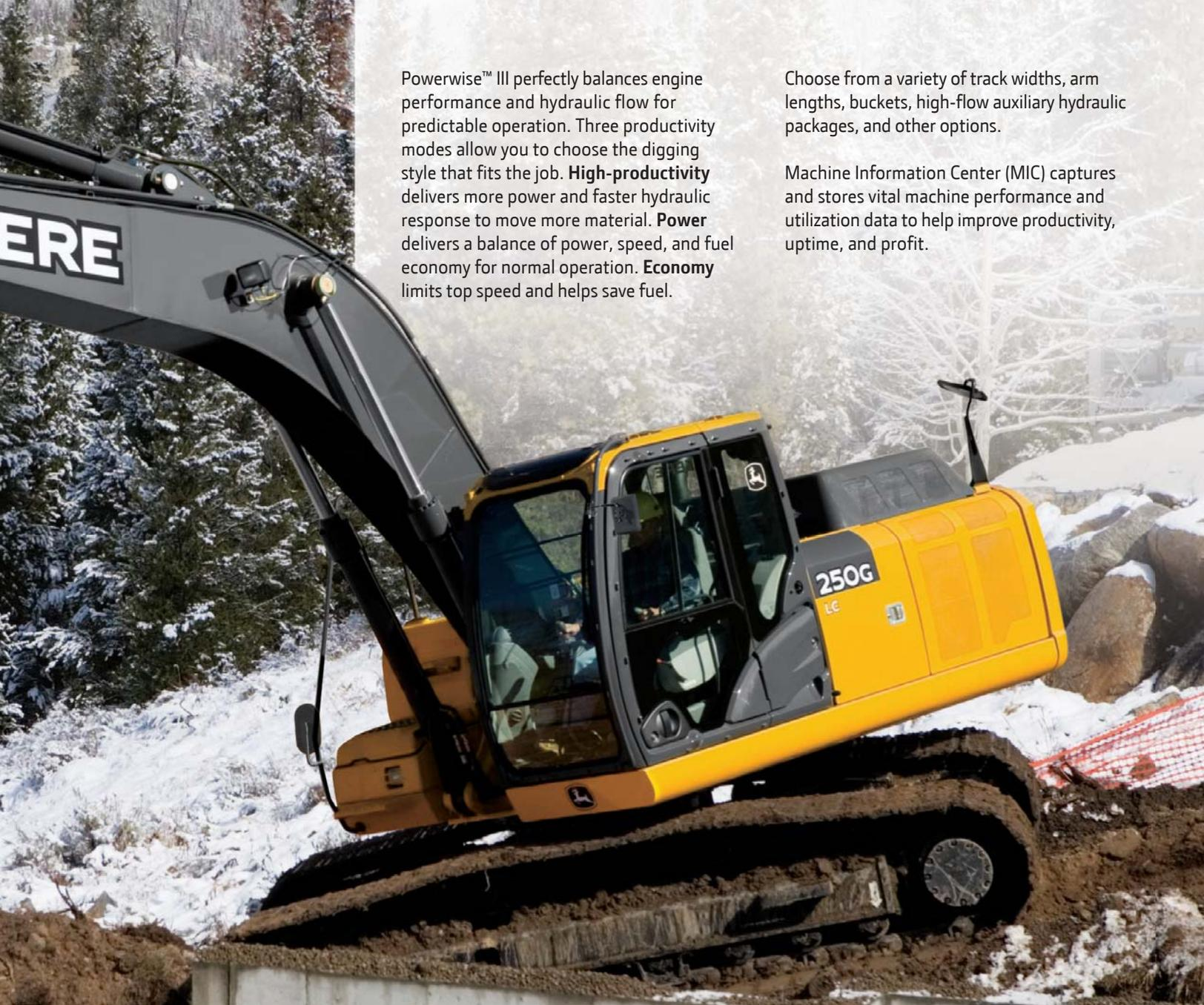
Powerwise™ III perfectly balances engine performance and hydraulic flow for predictable operation. Three productivity modes allow you to choose the digging style that fits the job. **High-productivity** delivers more power and faster hydraulic response to move more material. **Power** delivers a balance of power, speed, and fuel economy for normal operation. **Economy** limits top speed and helps save fuel.
