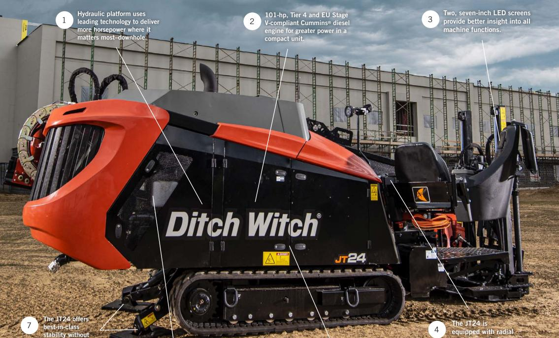
40-gpm, 1,200-psi mud pump offers increased fluid course from the mud pump to the swivel, funneling extra horsepower to the bit downhole
