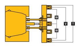
Heavy-duty parallelogram ripper, 5 shank pockets with 3 teeth 981 kg (2,163 lb.) 508 mm (20 in.) Weight Q Maximum Penetration 508 mm (20 in.) R Maximum Clearance Under Tlp S Overall Length, Lowered Position 1450 mm (57 in.) S<sup>I</sup> Overall Length, Raised Position
