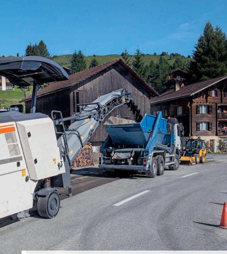
Powerful cold milling machine in the one-metre class for economical milling operations at a working width of 1.00 m or 1.20 m.
