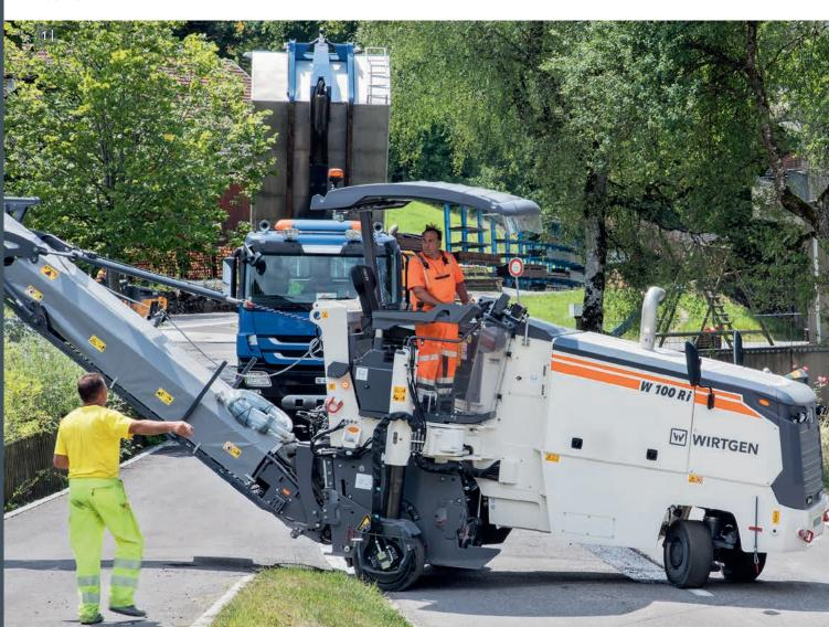
When pivoted in front of the milling drum, the right-hand rear wheel allows precise milling along obstacles such as kerbs or walls.
