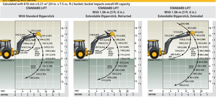
\*Indicates capacity is stability limited. Lift capacities are over end with stabilizers down and tires tangent to ground.
