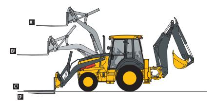
Calculated with 610-mm x 0.21-m³ (24 in. x 7.5 cu. ft.) bucket; bucket impacts overall lift capacity
