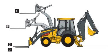
Calculated with 610-mm x 0.21-m<sup>3</sup> (24 in. x 7.5 cu. ft.) bucket; bucket impacts overall lift capacity STANDARD LIFT STANDARD LIFT
