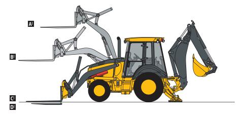
Calculated with 610-mm x 0.18-m³ (24 in. x 6.5 cu. ft.) bucket; bucket impacts overall lift capacity
