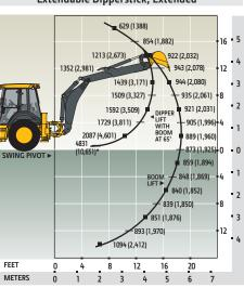
\*Indicates capacity is stability limited. Lift capacities are over end with stabilizers down and tires tangent to ground.
