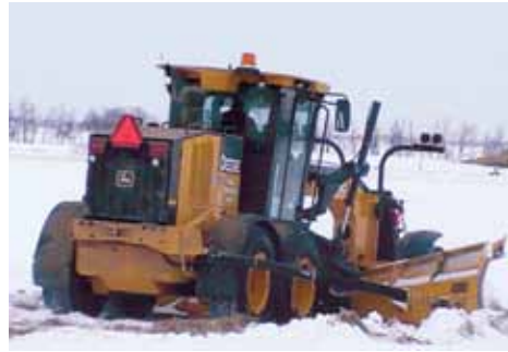
Brandt Snow Wing ready to go to work with the Deere 872GP Motor Grader.
