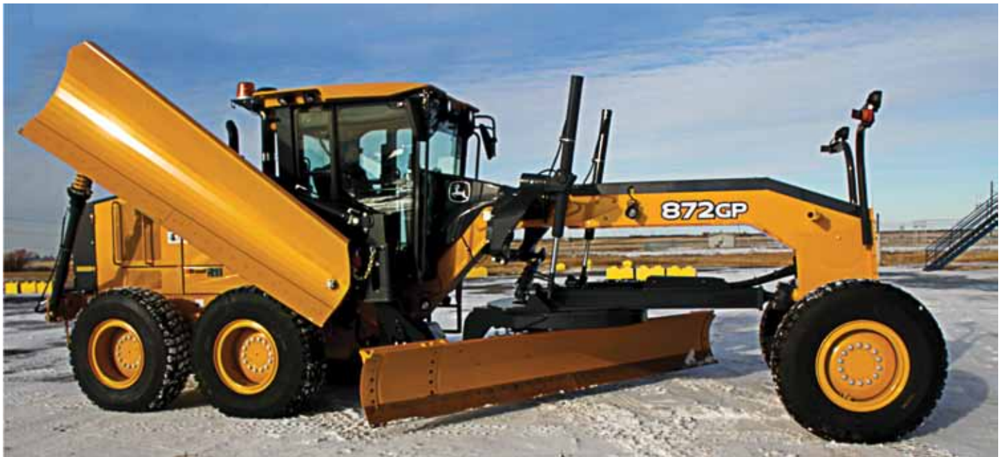
Brandt Snow Wing creates windrows in a field around Birch Hills, SK.
