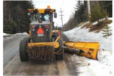
Brandt Snow Wing ditching a mountain road near Terrace, BC.
