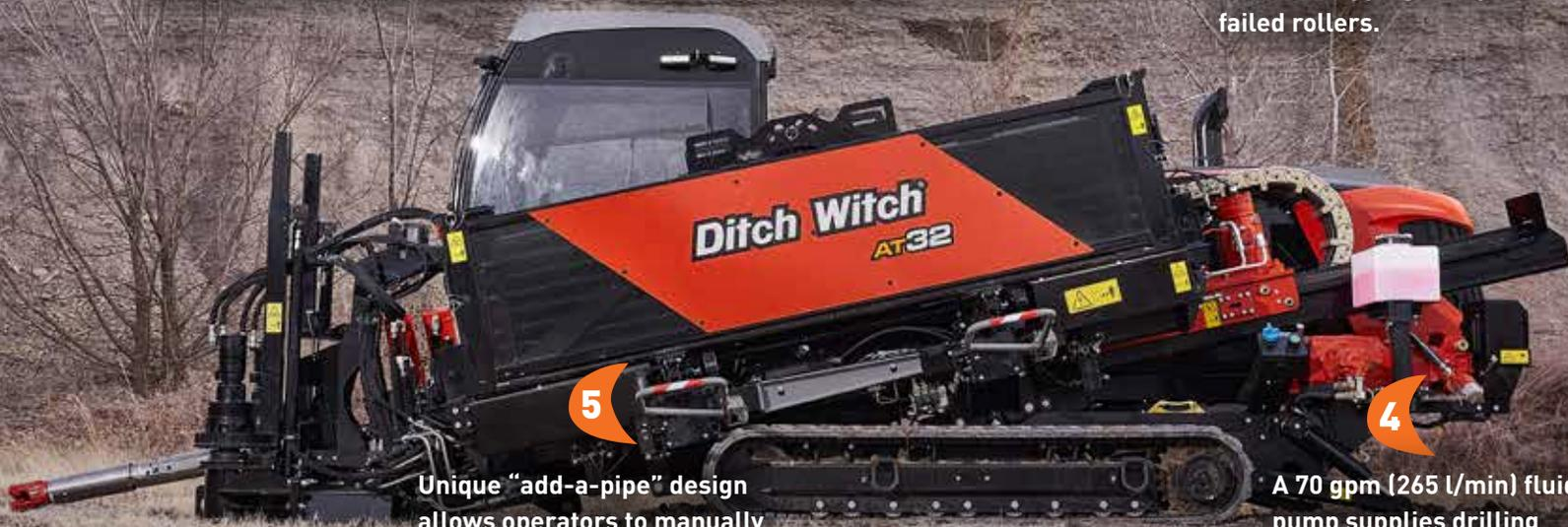
**5** Unique “add-a-pipe” design allows operators to manually insert additional pipe, improving productivity.
