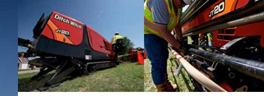
Auto-throttle feature saves fuel and reduces pollution by slowing the engine to idle after 15 seconds of inactivity; when you resume work, the auto-throttle engages.
